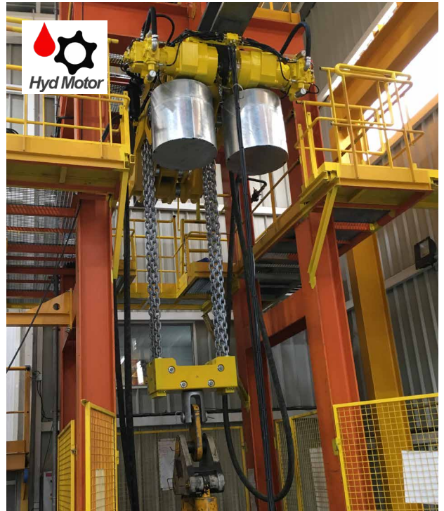
ULBS150 Factory Acceptance Test
