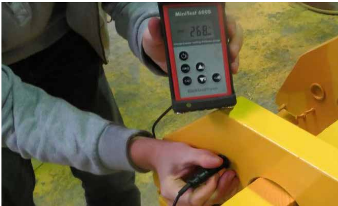
Dry Film Thickness Control
