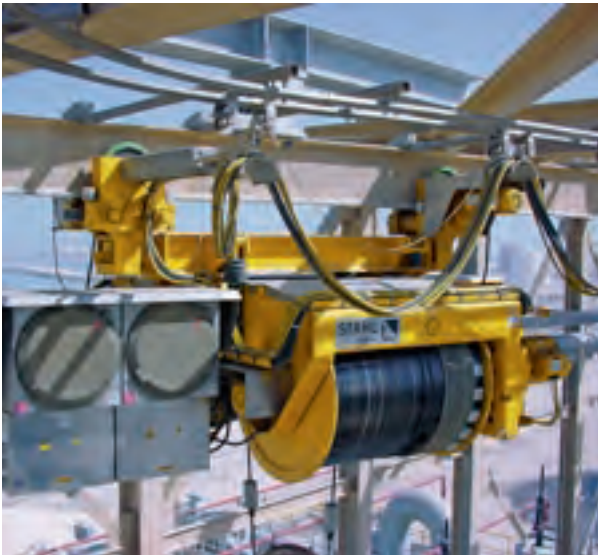
Maximum safety level 3B: normal operation even after rope breakage
